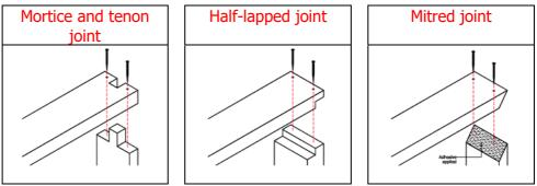
Figure 2. Head/Jamb jointing options
