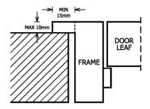
Figure 1. Frame option with integral architrave
