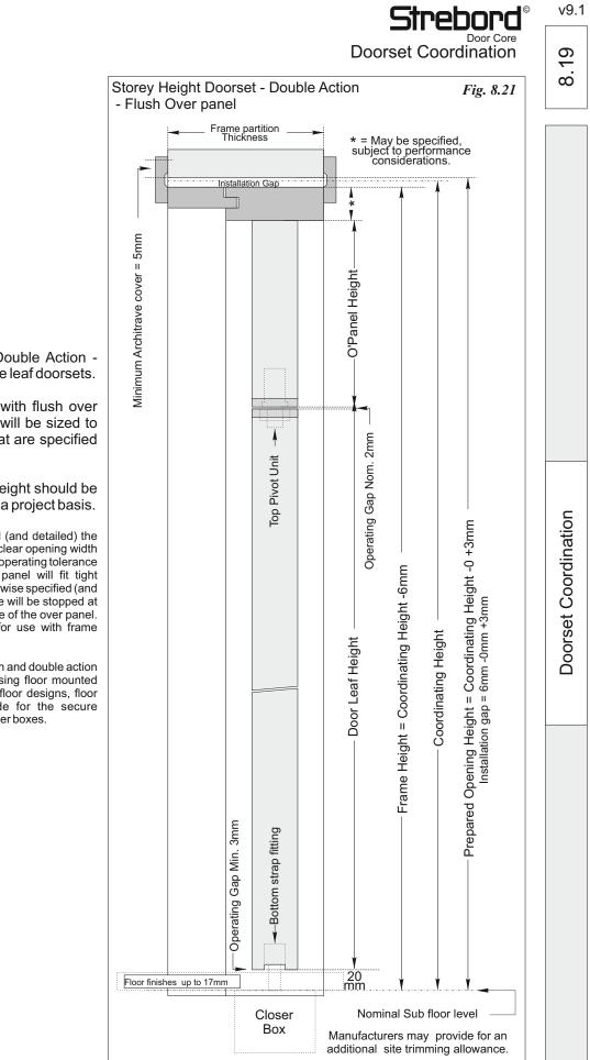
Storey Height Doorsets - Double Action - with Flush Over panel - Single leaf doorsets.
