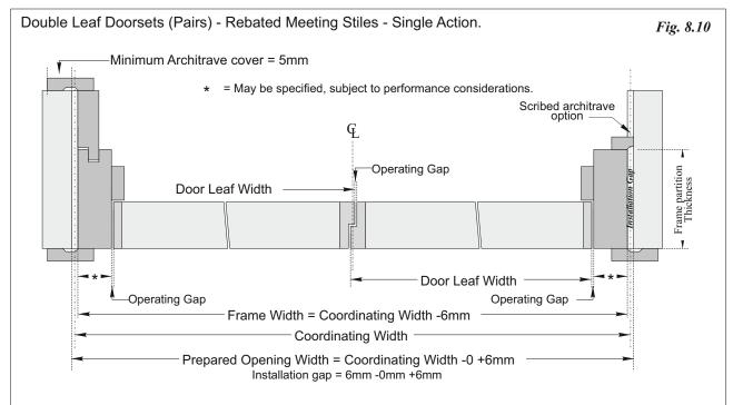
NOTE 1: The installation gap can be increased for frame designs using separate architrave subject to a minimum architrave cover of 5mm over the surrounding structure.
