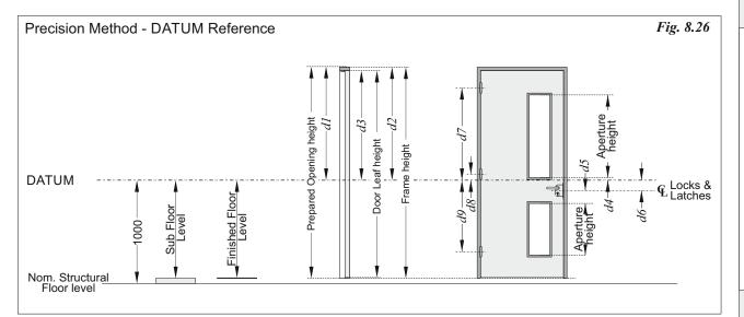
Using the Precision Method all work can be related to a common Project DATUM. For this example a DATUM height of 1000mm is indicated.
