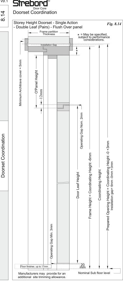
Storey Height Doorsets - Single Action with Flush Over panels - Double Door Doorsets (Pairs).
