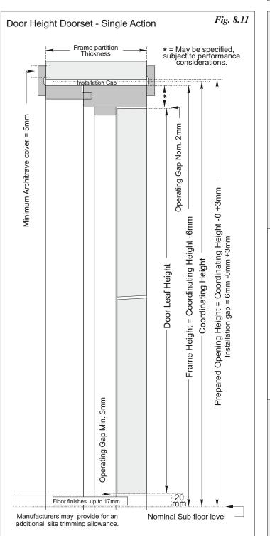
NOTE: The installation tolerance can be increased for frame designs using separate architrave subject to a minimum architrave cover of 5mm over the surrounding structure
