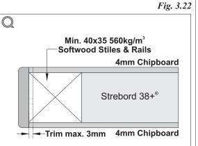
The Chipboard facings to be bonded to the core structure using an evenly applied cross linked PVA adhesive.
