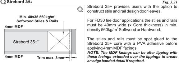
The MDF facings to be bonded to the core structure using an evenly applied cross linked PVA adhesive.
