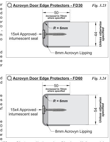
'intumescent' groove located within 100mm of the top and bottom edge of the door with the remaining fixings nominally equi-spaced between the top and bottom fixings, taking care to avoid conflicts with items of hardware. The fixings are then covered by the intumescent seal.
