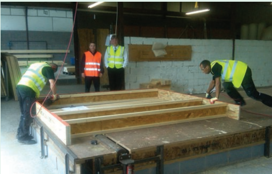
Available in a wide variety of depths and lengths and manufactured to match I-joists, LP SolidStart LSL Rim Board is ideal for use in floor cassette assemblies
